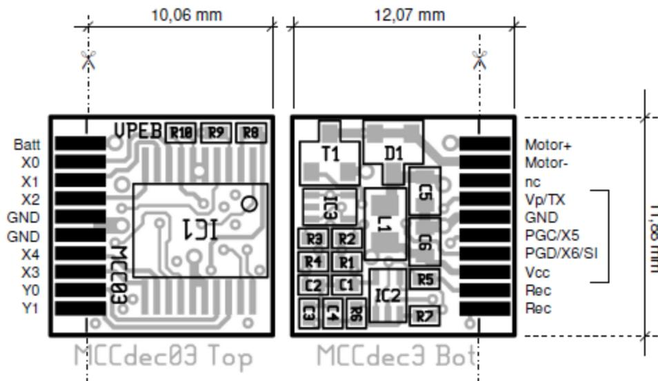
The connection diagram of MCCdec03 is almost equal to the one of MCCdec02. Just mark that MCCdec03 is one connection pad narrower than MCCdec02 (so in total 20 in stead of 22). At MCCdec02, the Motor-minus is located at the corner, at MCCdec03 that connection has "jumped over the Motor-plus". That pad was unused on MCCdec02. Further the double Vbat(+) is degraded to a single one.
