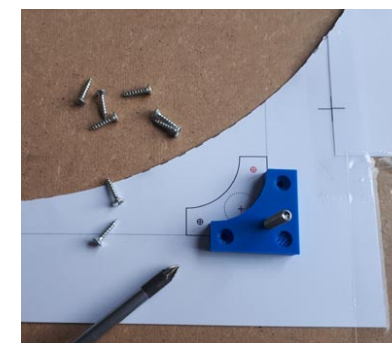
Figure 8: Mount the mounting block on the template. Only put in the screw in the red marked hole!
