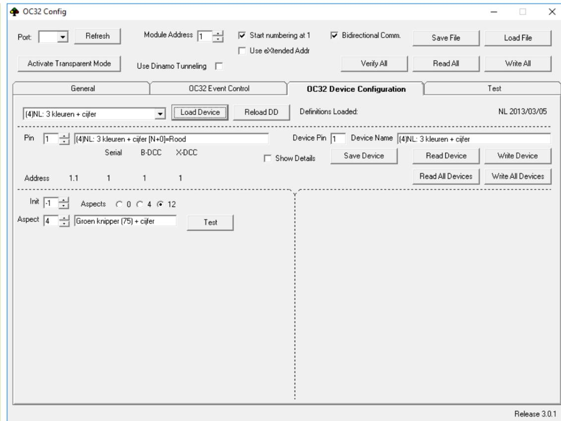
Fig 7: Configuring an NS signal with OC32Config
